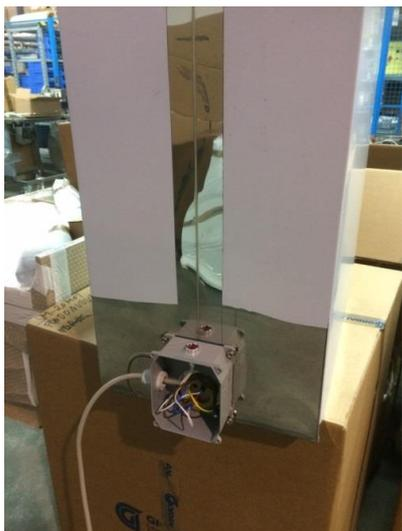
2. STACCATE I DUE CAVI A-B DALLA RESISTENZA DA SOSTITUIRE
